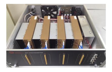
→ With two 2<sup>nd</sup> LOs in a parallel mode set-up, *two molecular lines (maximum 15GHz apart) can be simultaneously observable*. A single observation will enable us to get the data of 16 beams in 2 lines simultaneously, with the spectral bandwidth of ~60MHz.
